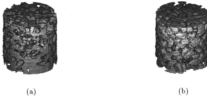
Figure 4: Rendering of the binary (a) porous phase (b) solid phase after 3-D reconstruction
